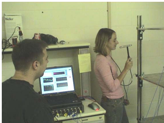
Figure 2. A LADSS student performing a modal test on a frame structure
