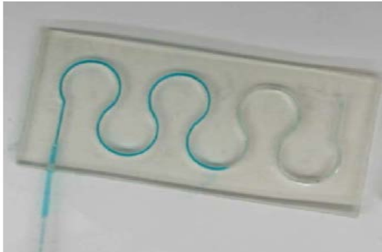
Figure 3: A dyed liquid is fills a serpentine microfluidic channel. The fluid flow is imaged with a CCD camera in the video mode. Each frame of the video is digitized, and (based on color differences) the flow front progression in each frame is determined.
