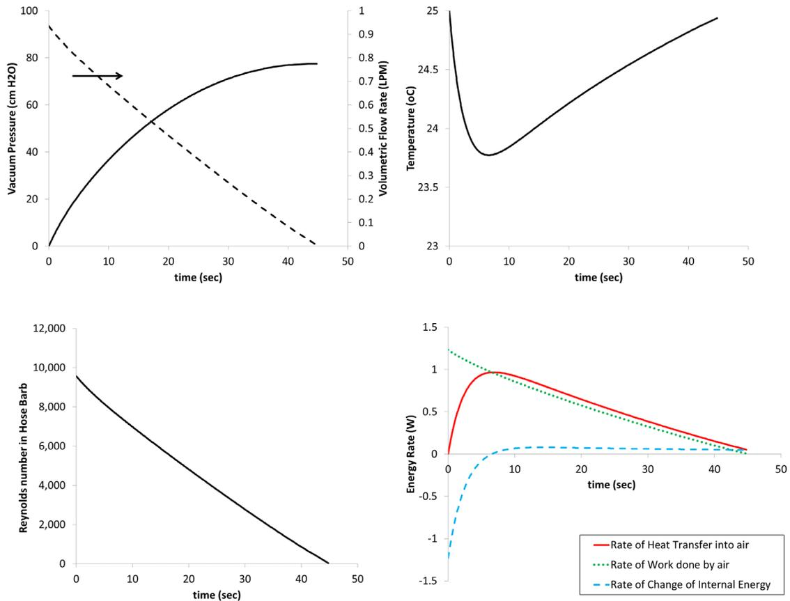
Figure 9. Results of a numerical simulation of a transient HVT event. Pressure (expressed as a vacuum in cm of H<sub>2</sub>O) and volumetric flow rate in top left, temperature in top right, Reynolds number in exit barb in bottom left, and energy rate terms in bottom right.
