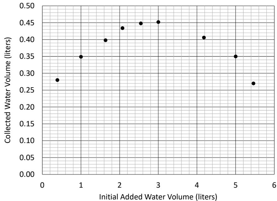
Figure 4. Sample plot of raw data taken from HVT1 during shakedown testing of Experiment I (Hydrostatic Vacuum Experiment). Collected water from test is plotted against the initial water charged in the system.
