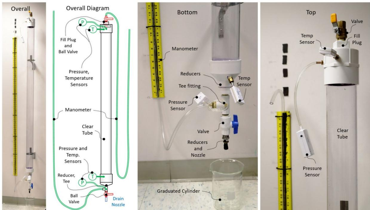
Figure 3. Overall (photo and diagram), bottom, and top sections of the second hydrostatic vacuum tube (HVT2). An additional manometer can be connected to the top ball valve to indicate the vacuum pressure as shown in the diagram (but it is not shown in the photos).
