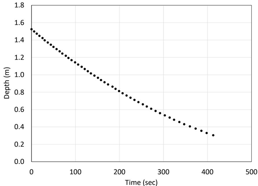
Figure 5. Sample plot of raw data taken from HVT1 during shakedown testing of the Draining Tank Experiment. Water depth is plotted against time.
