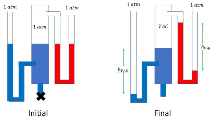
Figure 7. Initial and final illustration of a HVT with two manometers. HVT1.
