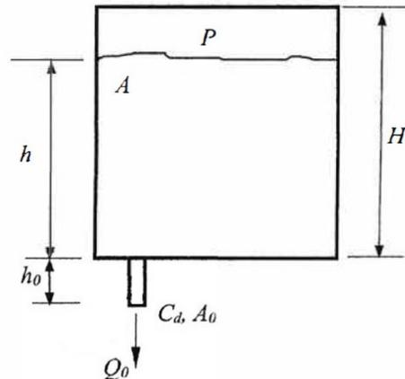
Figure 10. Geometry for differential equation draining homework problem.
