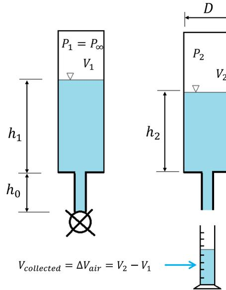
Figure 6. Schematic of experimental arrangement at the initial (1) and final states (2).
