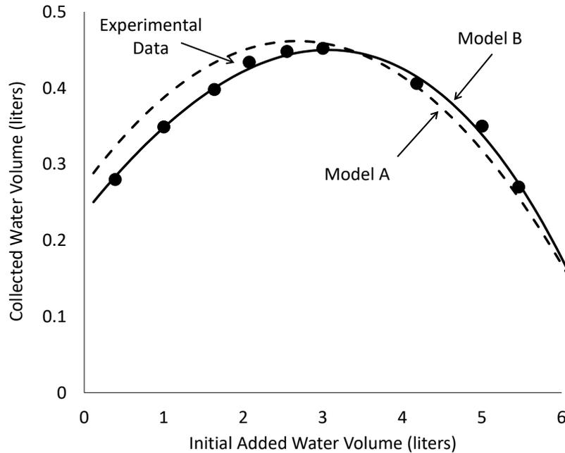
Figure 8. Model A (dashed) and Model B (solid) predictions with Experimental Data (filled data points) of Collected Water Volume vs. Initial Added Water Volume.
