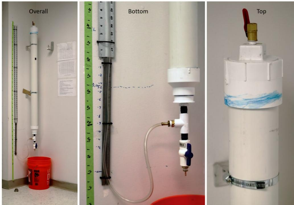
Figure 1. Overall, bottom, and top sections of the first hydrostatic vacuum tube (HVT1). Cost of materials was approximately \$50 and all parts were purchased from a local hardware store
