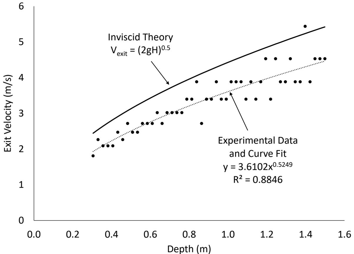
Figure 9. Exit velocity plotted against water depth for the draining tank. A power law fit is applied to the data (informed by theory) and the prediction obtained by inviscid theory (Bernoulli's Law) is also shown.
