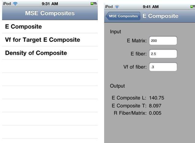
Figure 11. Unidirectional Composite Calculator for E and Density
