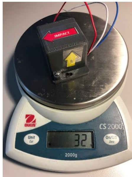
Figure 8 Photo of DUT weight testing.
