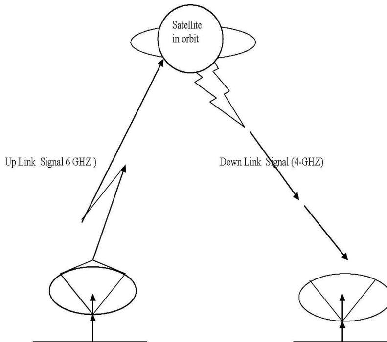
The above setup shows how information can be transmitted via satellite in orbit at about 23,000 miles from earth.
