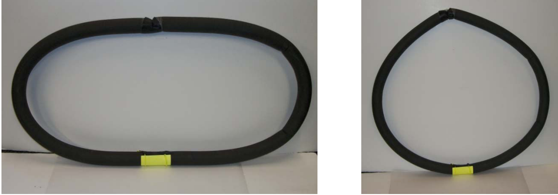
Figure 7. Foam Tank Tread / Non-slip Wheel Demonstration of Instantaneous Center of Rotation
