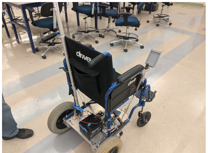
Fig. 3. The Customized Wheelchair after Motor and EMOTIV Integration
