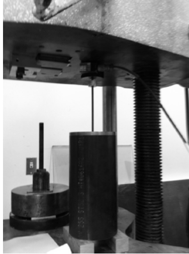
Figure 18 – Piston-Cylinder Friction Testing in an Instron Machine
