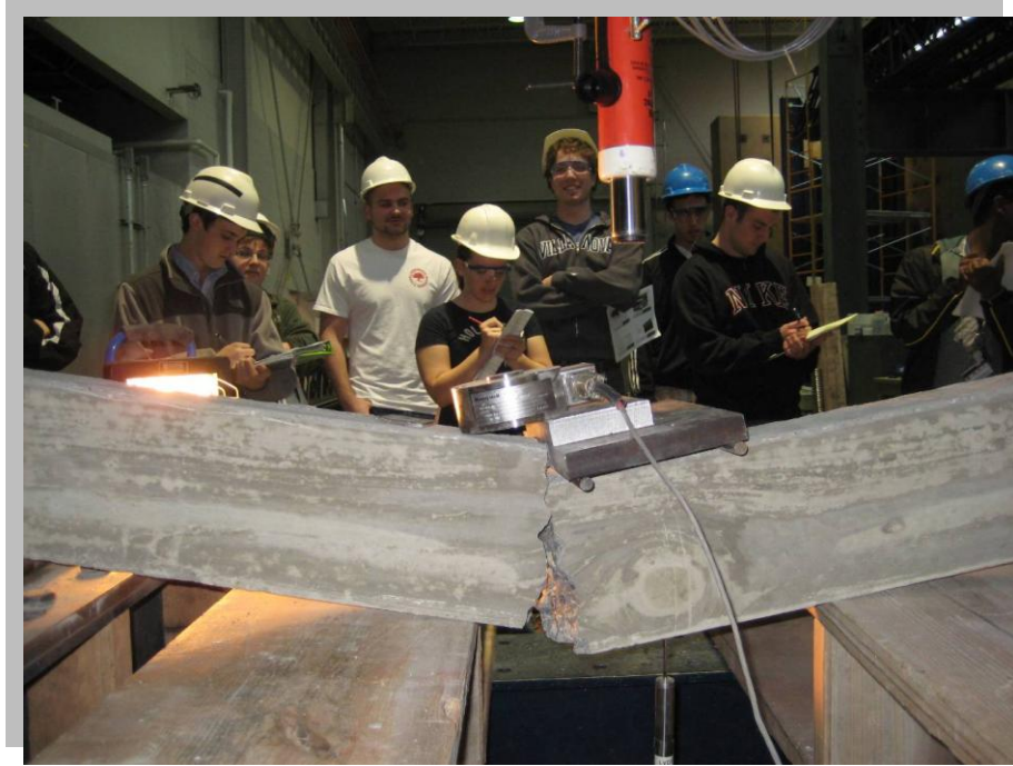
Figure 2. Students test a reinforced concrete beam and note their observations.
