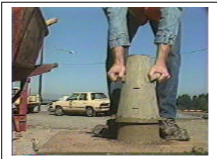
Lifting slump cone
