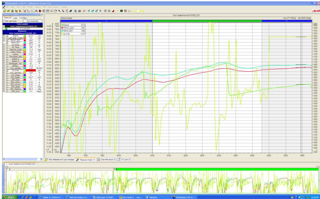
Figure 8. Test trace of front and rear EGTs, engine rotational speed and Air-to-Fuel ratio
