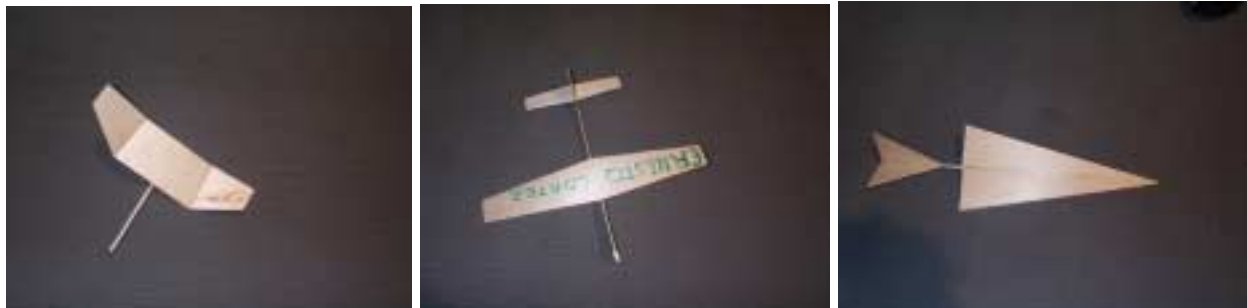
Fig. 6: Balsa Wood glider design concepts: flying wing, monoplane, delta wing (from left to right)
