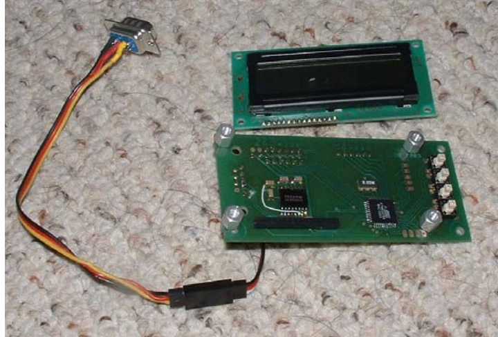
Figure 2: Microcontroller Autopilot Developed by the Author
