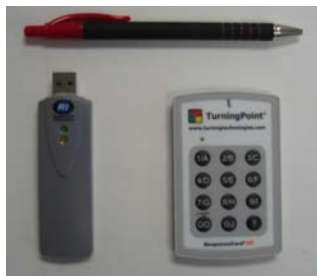
Figure 1. Turning Technologies TurningPoint ResponseCard ® RF wireless response system. The system includes a universal serial bus (USB) receiver and 25 response cards. The pen is shown for size reference.
