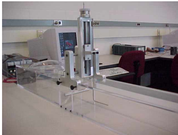
Figure 2. Picture of table top wind tunnel and probe assembly showing the test cylinder mounted on the test plate.
