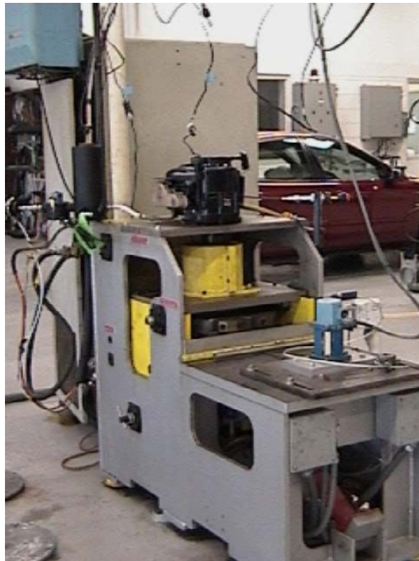
Figure 2: Photograph of the dynamometer set-up with one of the engines mounted for testing.
