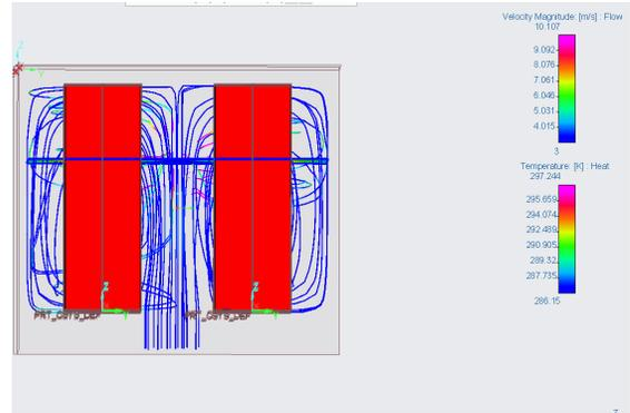
Fig. 7. Air flow trajectory of cold aisle containment Type 04
