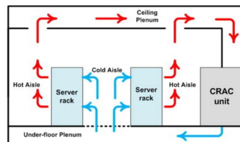
Fig. 1. A basic hot aisle/cold aisle raised-floor data center [5]
