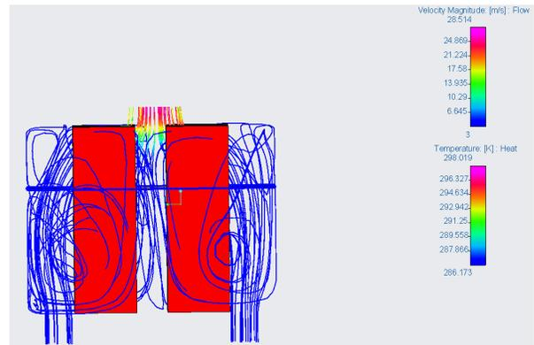
Fig. 8. Air flow trajectory of hot aisle/cold aisle Type 02 model
