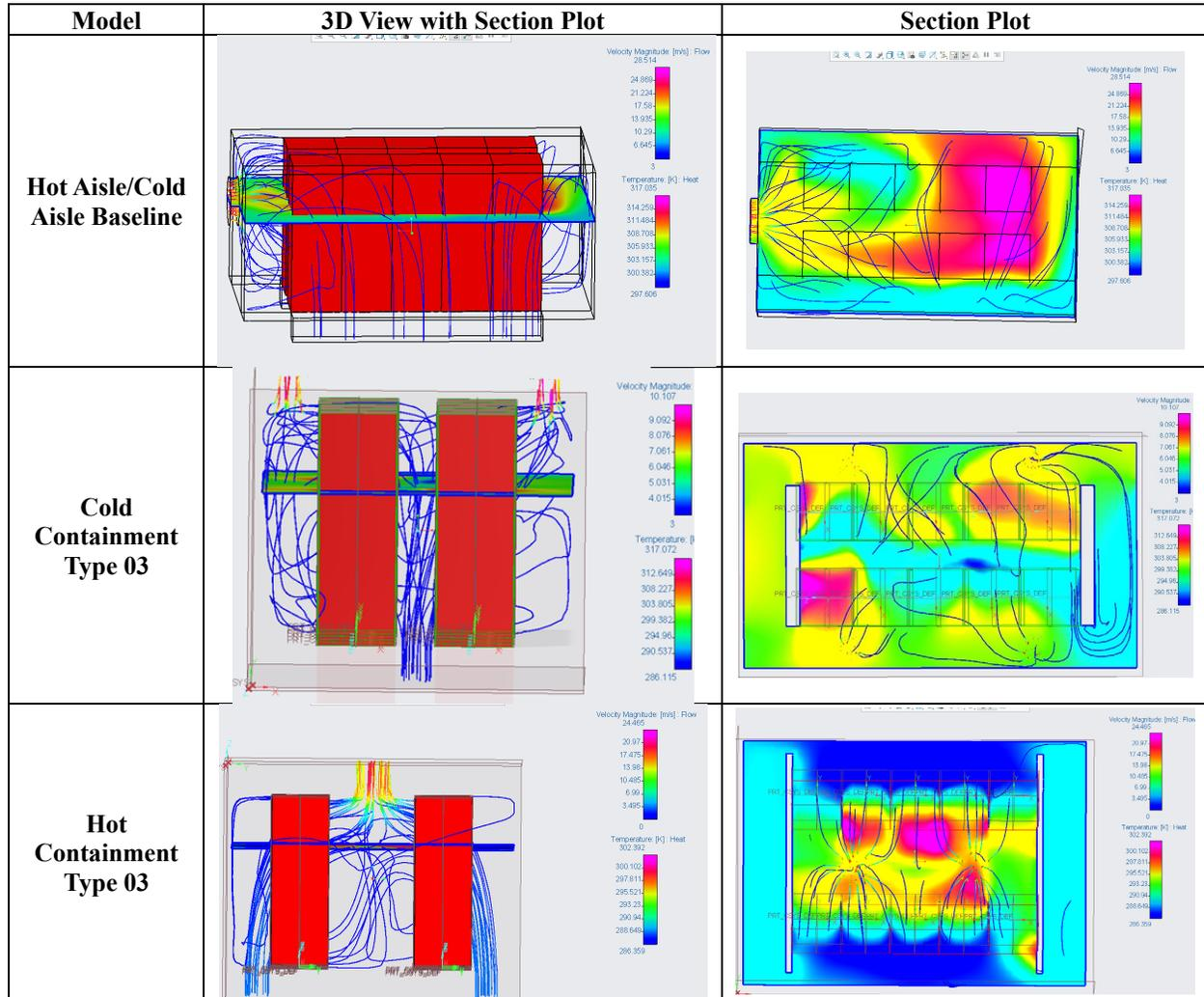
Fig. 4. 3D Views and section plots for three models
