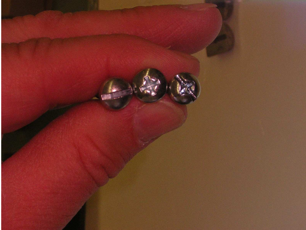
Figure 2: Slot, Phillips, and Combination Screw Heads
