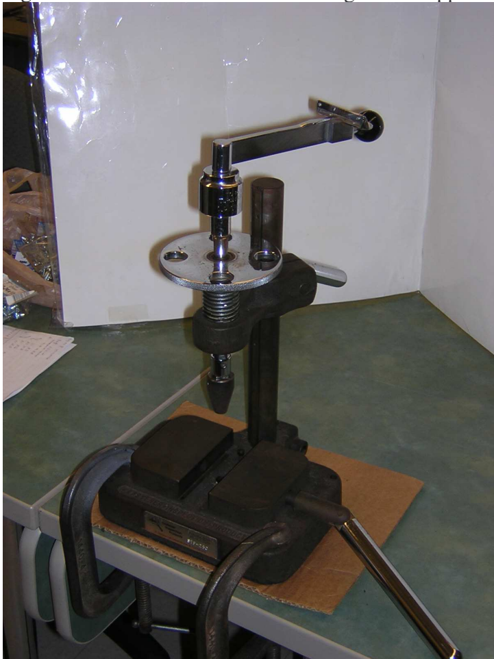
Figure 5: Torsional Strength Test Apparatus
