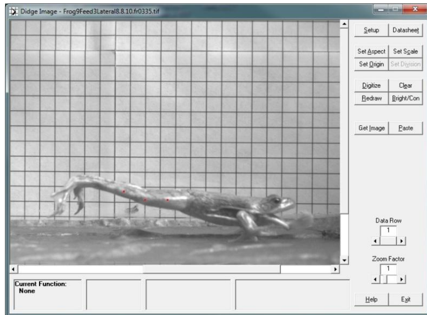
Figure 3: Screenshot of the Didge image digitizing software used to calculate changes in joint angle.
