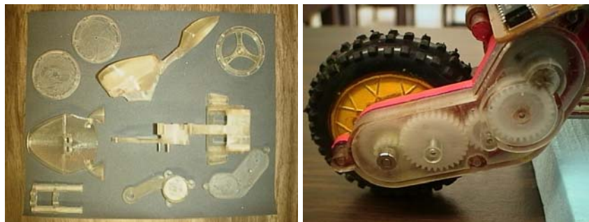
Figure 4: The physical prototype was made using SLA-stereo lithographic technique. SLA is a common rapid prototyping technique, which produces acrylic and epoxy parts. The unpainted parts are shown to the left. The gearbox housing and transmission is shown unpainted to the right
