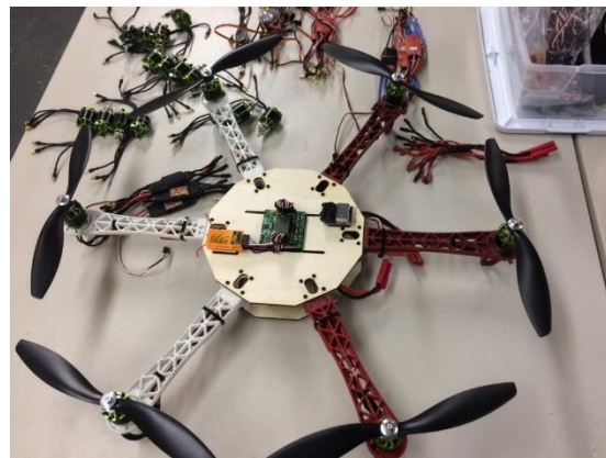
Figure 5. Adapt challenge: Building a hexcopter using laser cut assembly board
