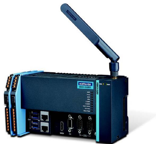
(b) AMAX-5580 with EtherCat modules (Courtesy of Advantech Co. Ltd.)
