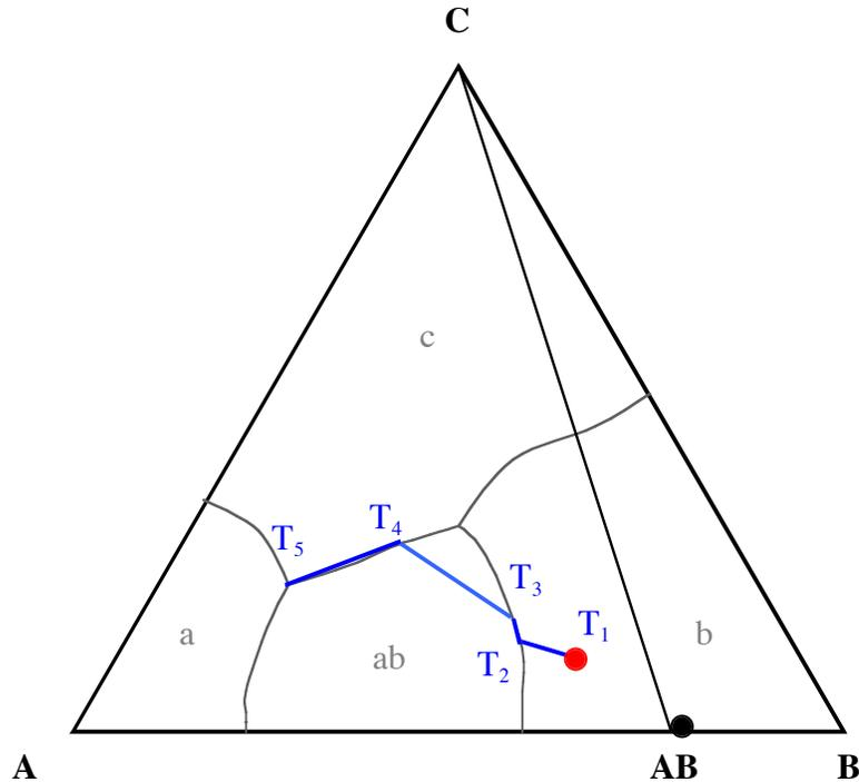
Figure 3. A two dimensional projection of a three component phase diagram with an incongruently melting binary compound, AB. The composition of the isopleth is 29%A, 60%B, and 11%C (dot at  $T_1$ ) and its crystallization path proceeds from  $T_1$  to  $T_2$  to  $T_3$  to  $T_4$  and ends at  $T_5$ .
