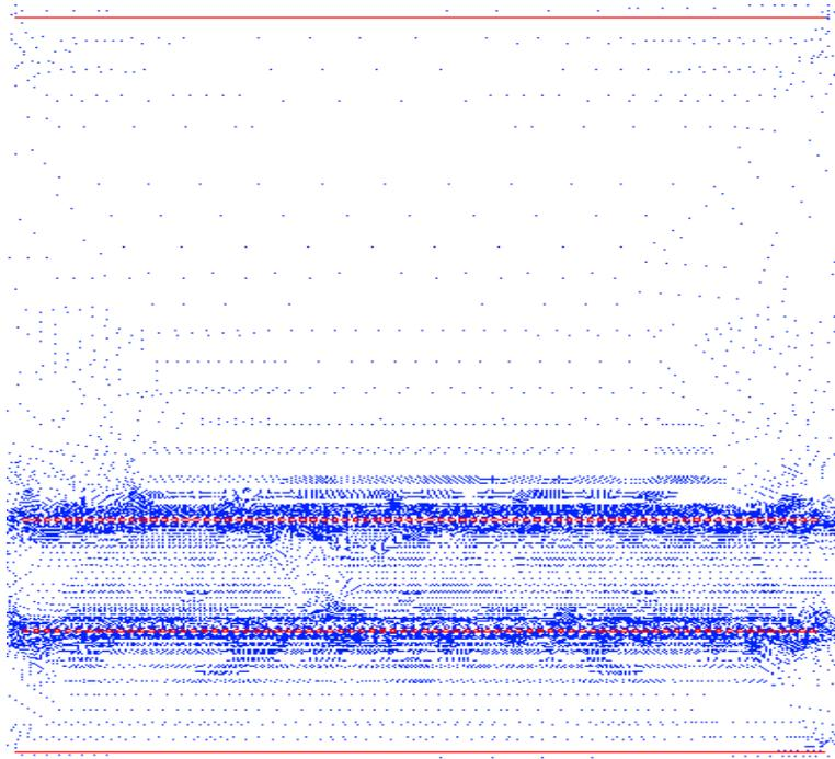
Figure 2b. The electric field lines for a double GEM showing the drift, amplification, and collection regions. Notice the concentration of the Electric field within the GEM holes. The Mylar, the GEM and the PCB are shown.
