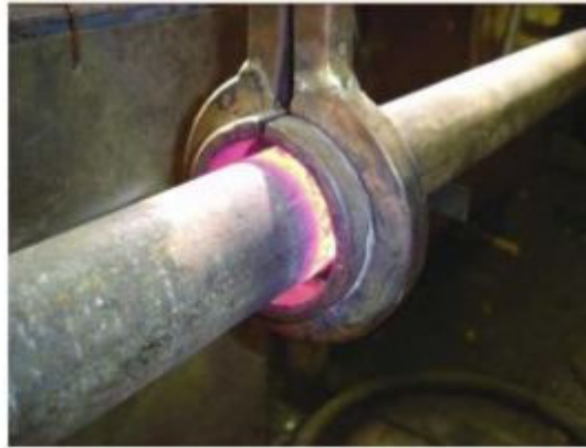
Induction coil around the pipe during the induction welding operation
