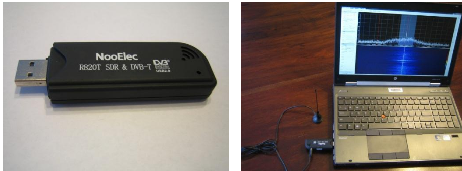
Figure 1: The RTL-SDR based on the R820T tuner and the mobile studio
