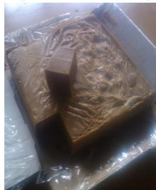
Photograph-11: Cutting unmolded soap into bars
