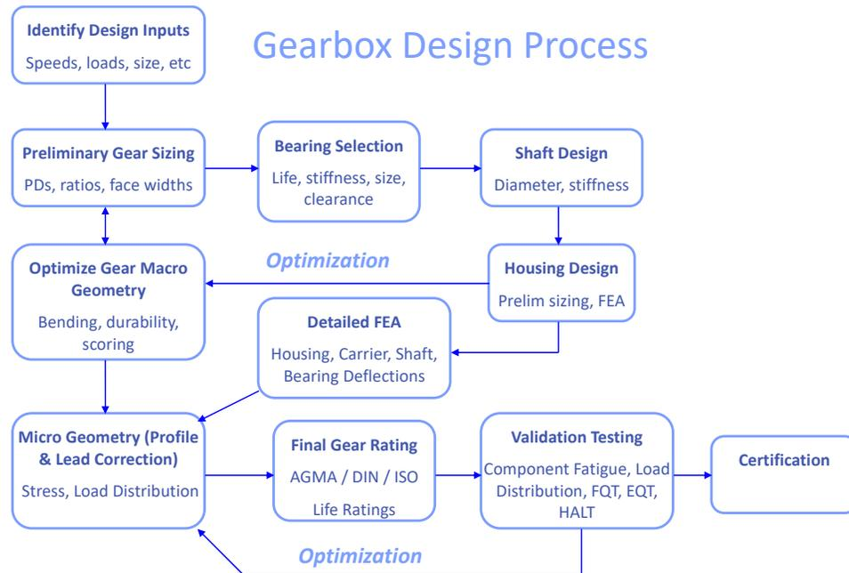
**Figure 3.** The Typical Gearbox Design Process
