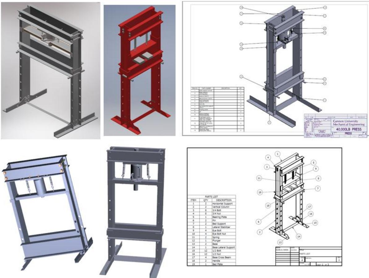
**Figure 2.** Examples of student work for 20-ton shop press. Students must create CAD assembly model, detailed assembly drawing with BOM and detailed drawings for each critical component.
