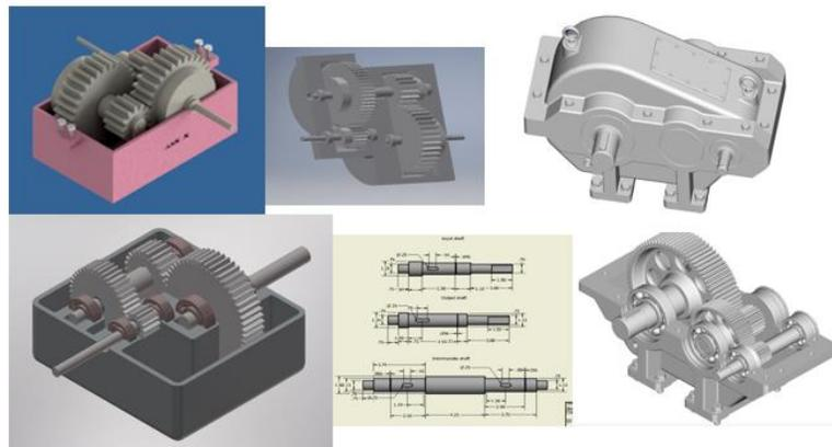
**Figure 4.** Student examples of speed reducer solid model.
