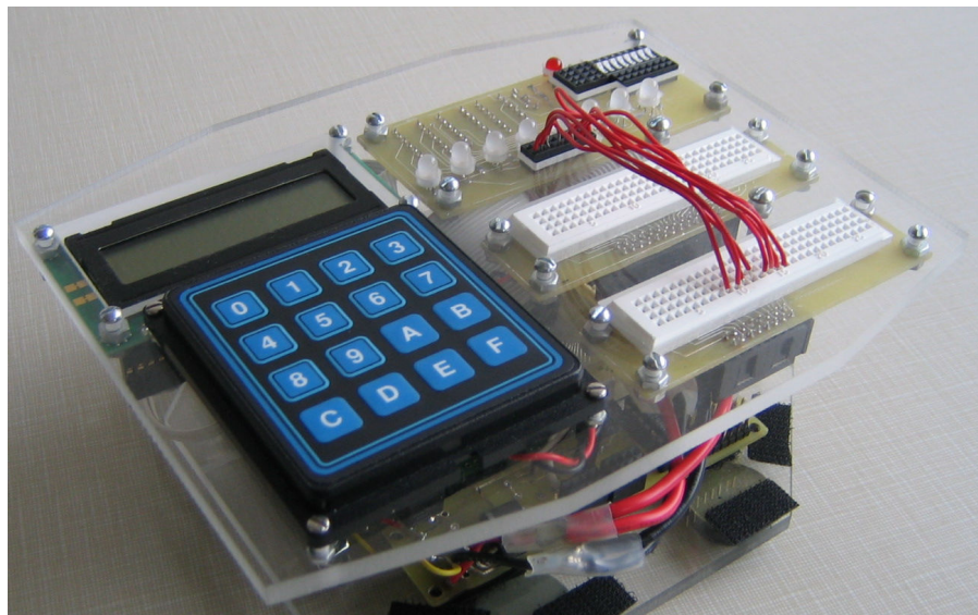
Figure 2: Top plate (with center-plate attached)
