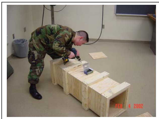
Figure 6. Construction of the soil-containment box used at the firing ranges.
