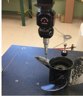
Fig. 1- CMM setup for geometry detection.
