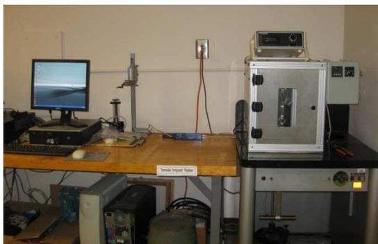
Figure 1: The tester and set up. Tensile load is applied from the bottom.
