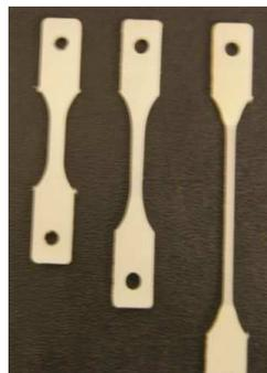
Figure 8: A typical sample, from left to right: undeformed, partially and then extensively crept.
