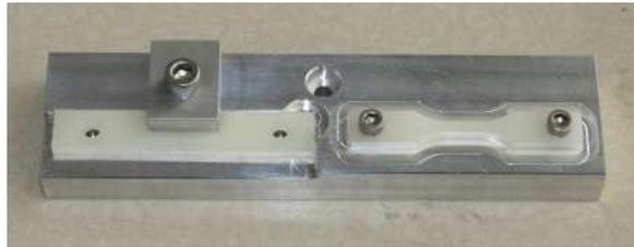
Figure 4: The CNC milling jig to manufacture the dog bone specimens.
