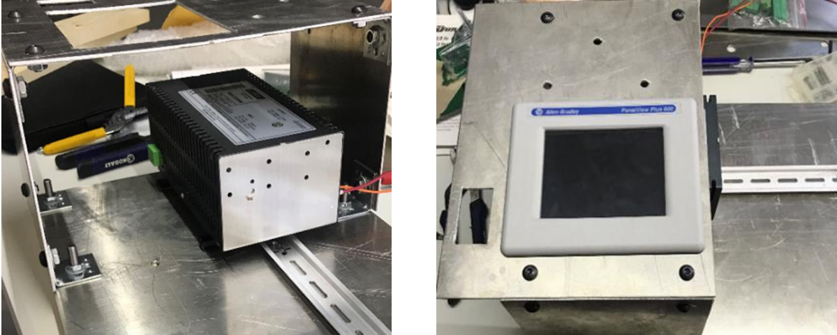
Fig. 6. Mounting the power supply and the HMI.
