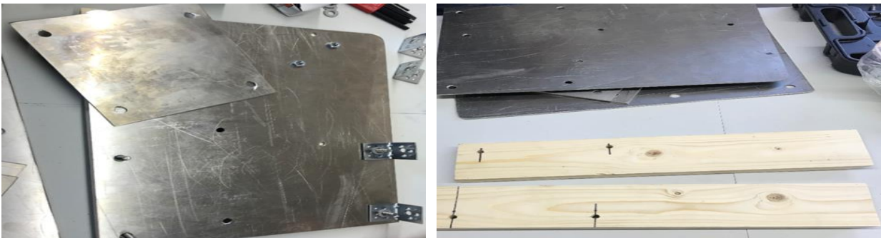
Fig. 2. The metal sheets and plywood base for the trainer's case.
