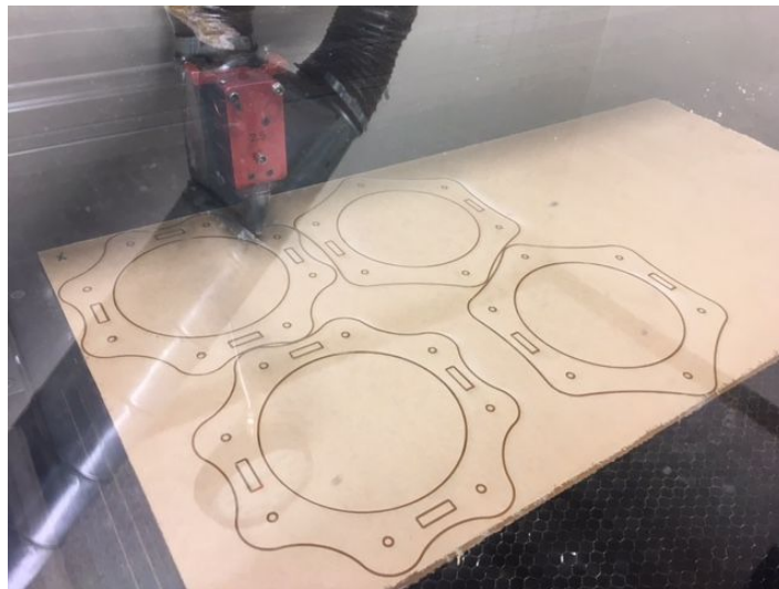
Figure 3: Student designed pieces of plastic being fabricated on the laser cutter.
