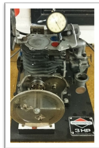
Figure 2. Cutaway one cylinder spark ignited engine
