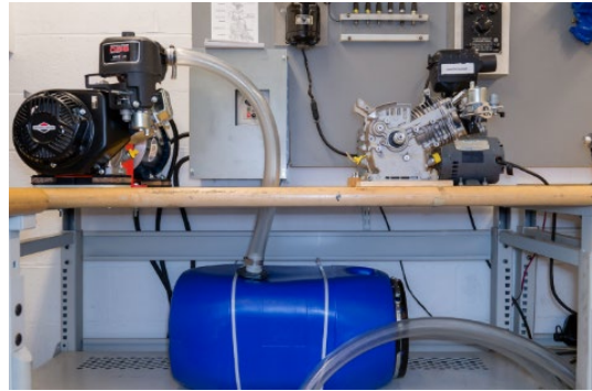
Figure 11. Setup to measure volumetric efficiency
