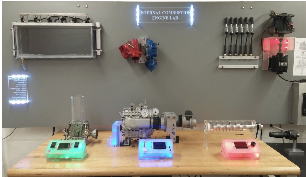
Figure 3. Air and fuel induction setups and spark generation.
