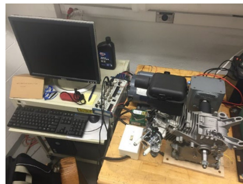
Figure 10. Setup to measure mechanical efficiency
