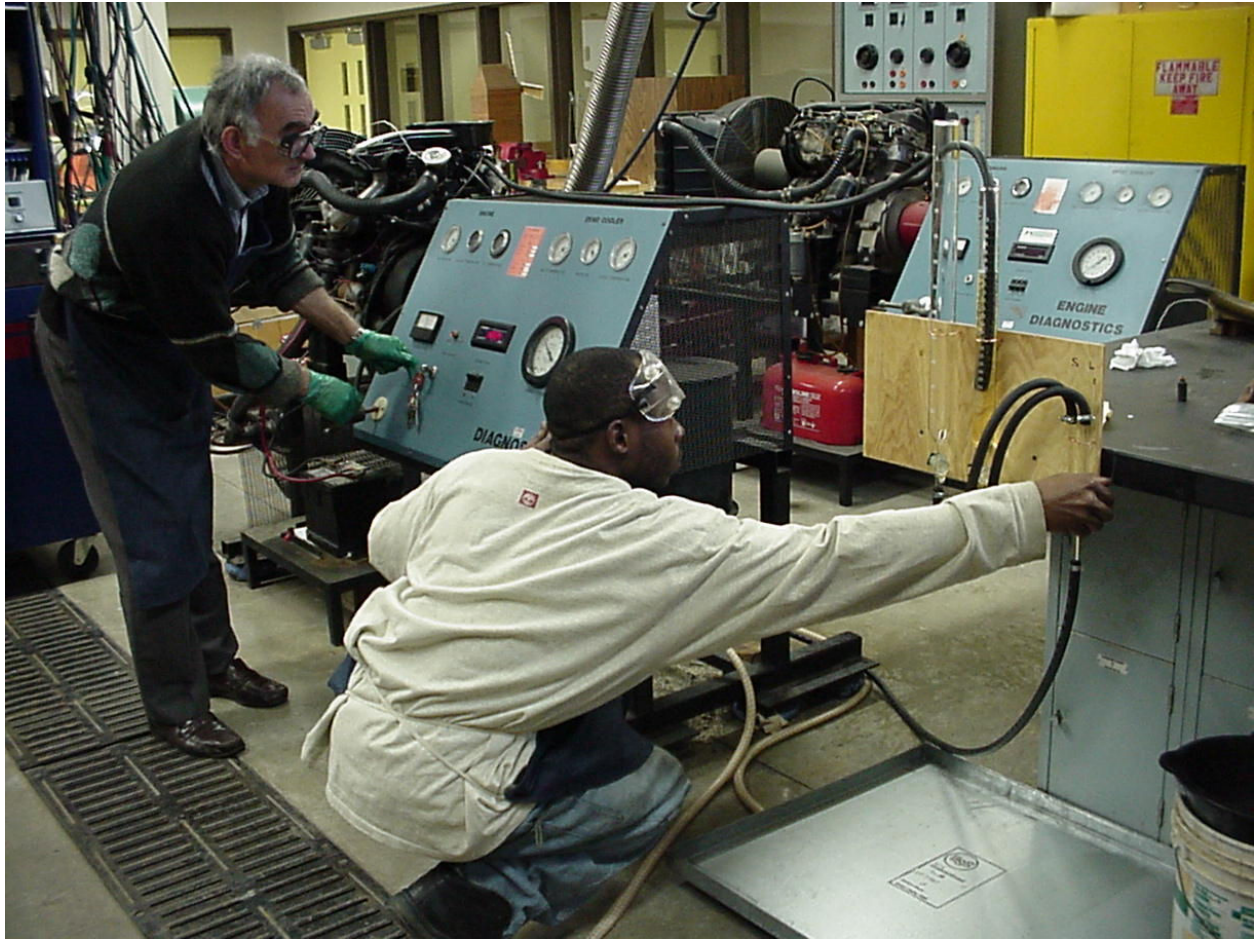
Figure 5. The Dynamometer and The Volumetric Fuel Measuring System.
