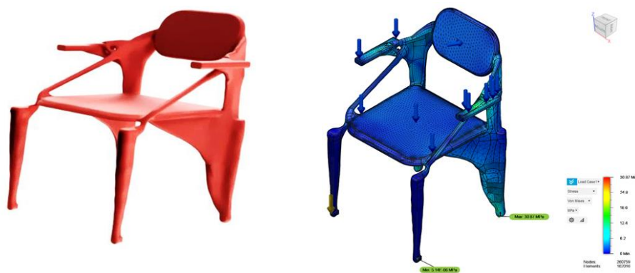
Figure 3. Final Design and Static Simulation
