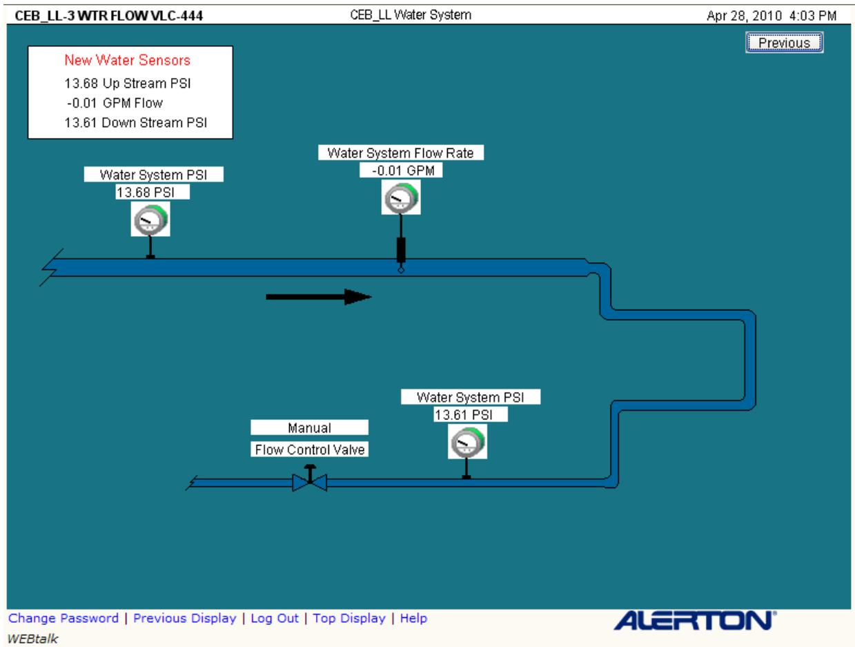
Figure 4.0, Graphical display of the instrumented pipe.
