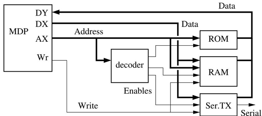
Figure 8: System with Memory and One Device
