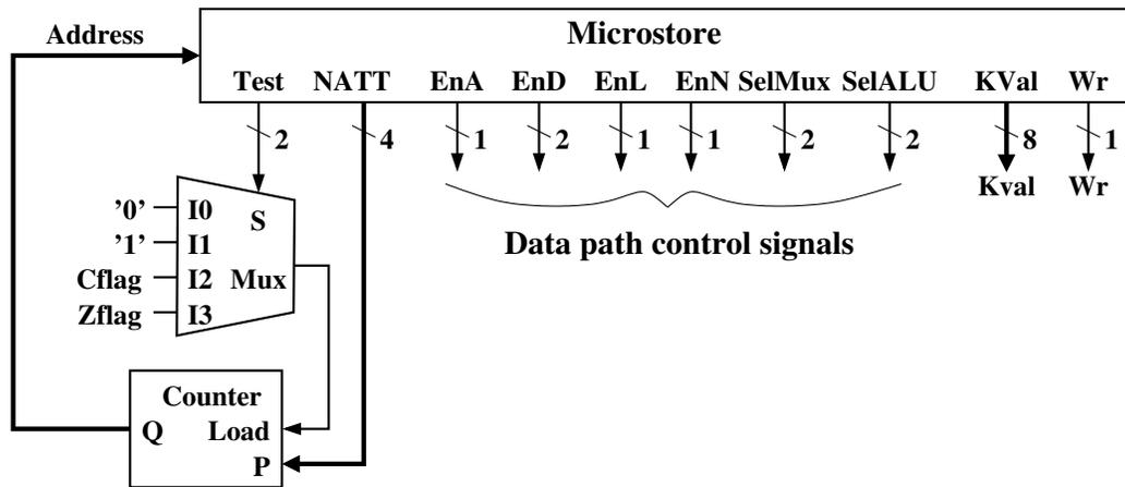
Figure 4: Microcode-Based Controller
