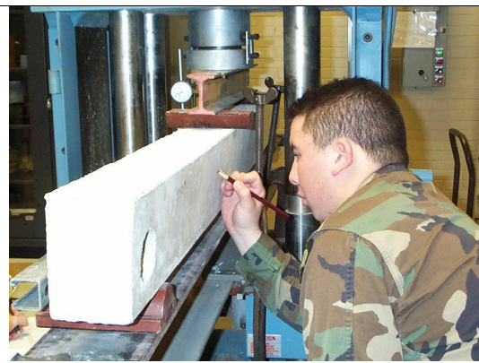
Figure 12: Cadets Identify the Crack Pattern on the RC Beam
