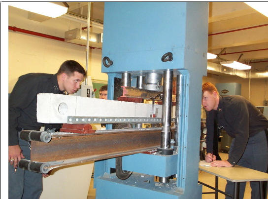
Figure 9: The Test Set-Up For The Reinforced Concrete Beam
