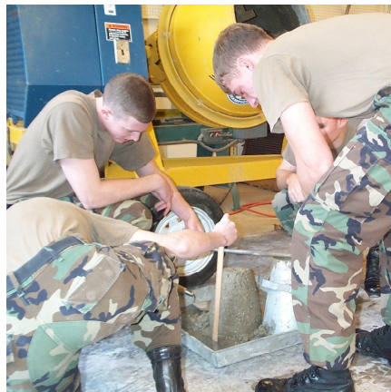
Figure 1: Cadets perform a slump test to evaluate the workability of their concrete batch
