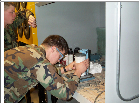
Figure 11 : A Sulphur Cap is Applied to the Concrete Test Specimen
