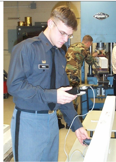
Figure 8: A Pachometer is Used to Determine the Location of the Steel Reinforcement
