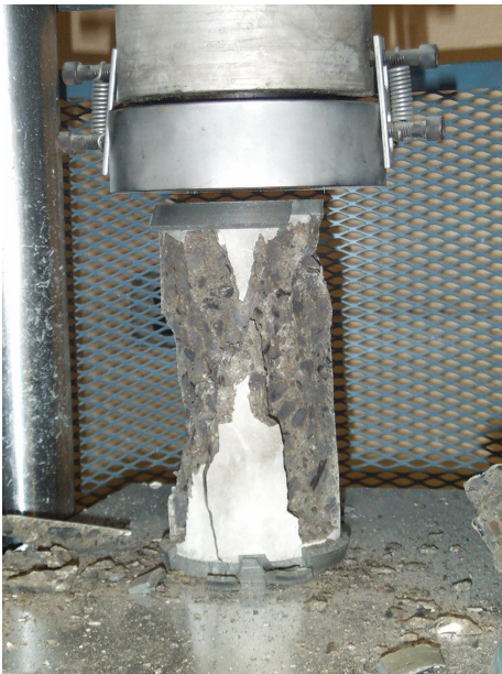
Figure 3: A 4"x8" Concrete Specimen Being Tested For Compressive Strength
