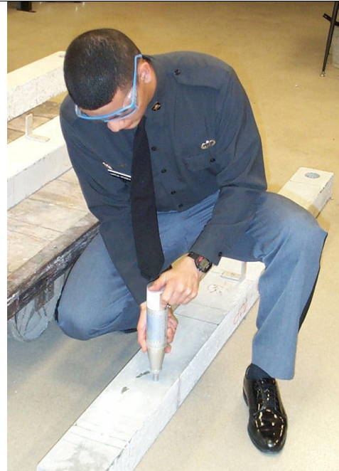
Figure 6: A Schmidt Rebound Hammer Tests the Concrete Strength
