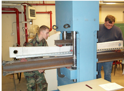
Figure 14: Cadets Observe That Reinforced Concrete Behavior Can Be Quite Ductile
