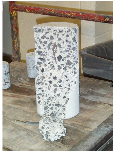
Figure 4: The Embedded Strain Gage Can Be Observed in the Crushed 6" by 12" Concrete Specimen
