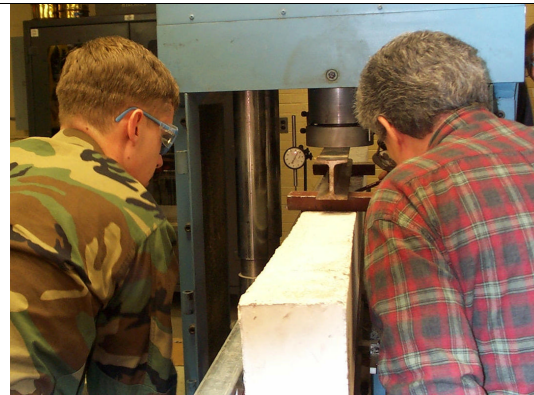
Figure 10: A Dial Gage Records the Deflection at the Center of the Beam
