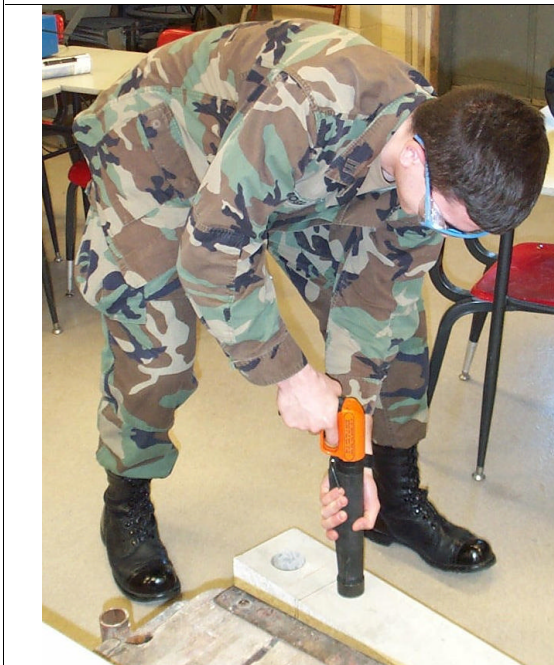
Figure 7: A Cadet Fires a Windsor Probe Into the Concrete Beam
