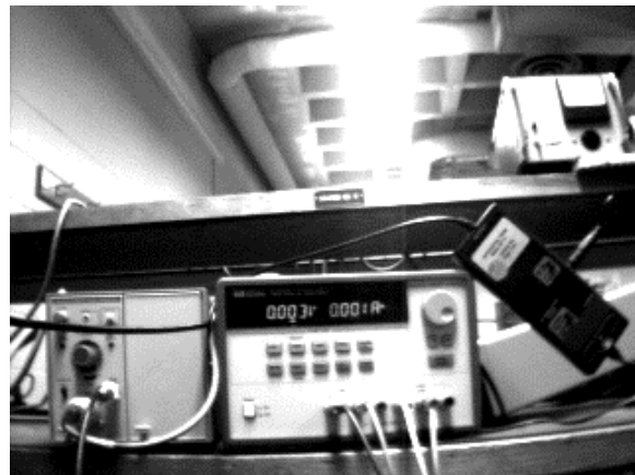
Fig. 10. The Current Amplifier, Power Supply and Voltage Isolator
