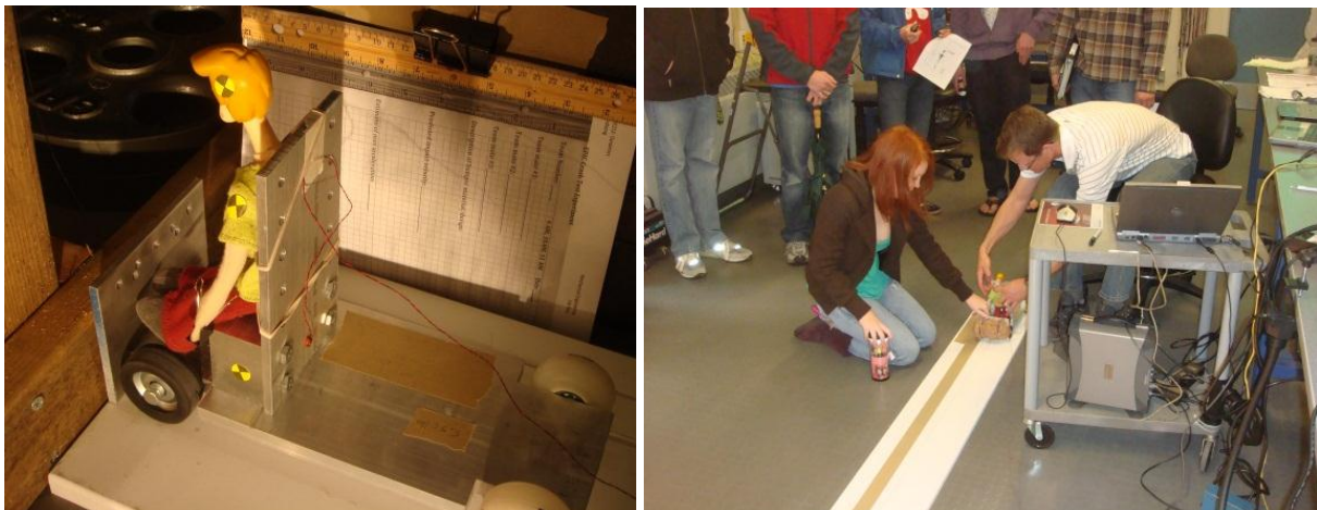
Figure 4. Photo of crash test vehicle and dummy on track at impact barrier (left) and student setting up experiment (right)
