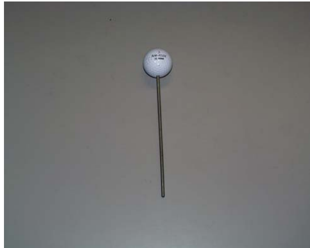
Figure 3: Golf ball mounted for insertion in two component force balance.
