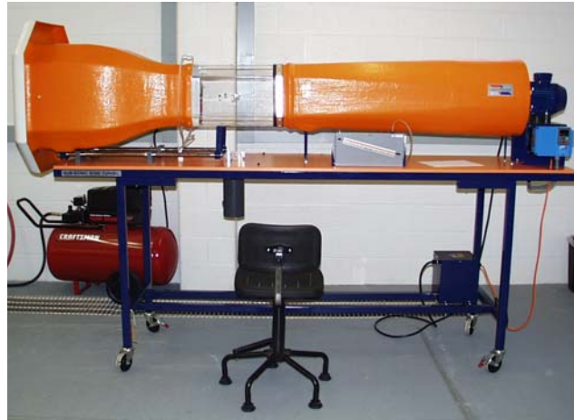
Figure 2: University of Kentucky, Paducah model wind tunnel used for classroom instruction.
