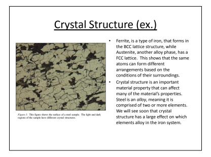
Fig. 1b: Slide with a specific and practical case of how crystal structure can affect microstructure, illustrating the basic information presented in Fig. 1A with an example involving steel.
