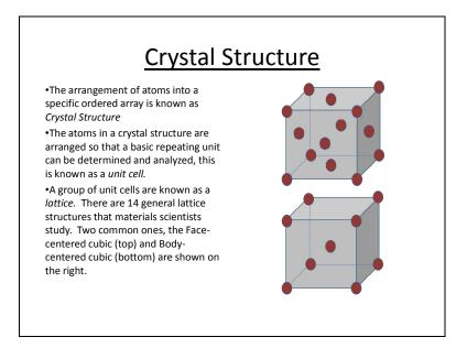
Fig. 1a: An example of a slide contained in the presentation given to materials science and engineering freshman. An understanding of the fundamental concept of crystal structure is essential for students, as it affects the properties of nearly all metals, alloys, technical ceramics and electronic materials.
