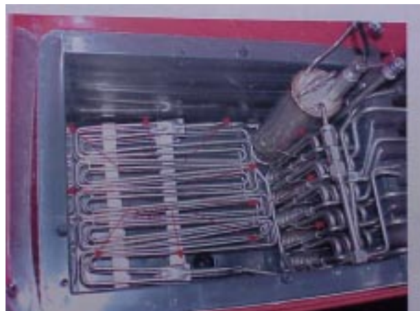
Figure 2. Cold Carbonated Beverage Dispenser Showing Ice Bank Tank with Product Lines.
