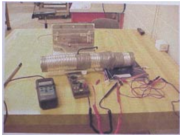
Figure 4. Assembly to characterize the performance of a computer case fan.
