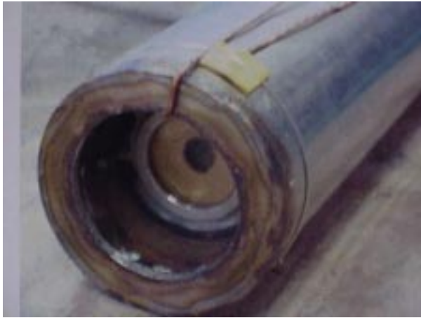
Figure 5. In-furnace video camera housed in water-cooled jacket.
