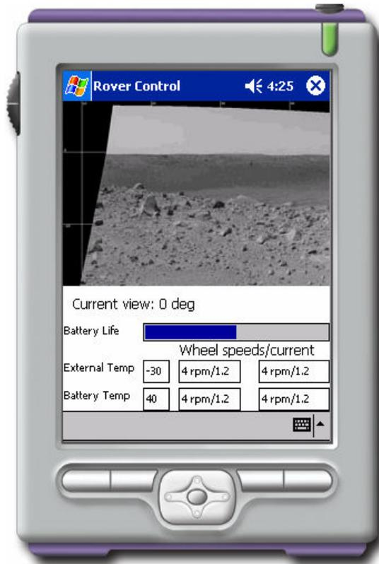
A handheld or portable device will be used as a base station. The digital images from the rover cameras will be displayed. The status of the rover, including camera viewing angle, battery life, external temperature, wheel rotational speed, current, etc. will also be displayed. A human operator can also use this device to send commands to the rover.
