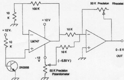
Figure 3: Circuit for temperature measurement
