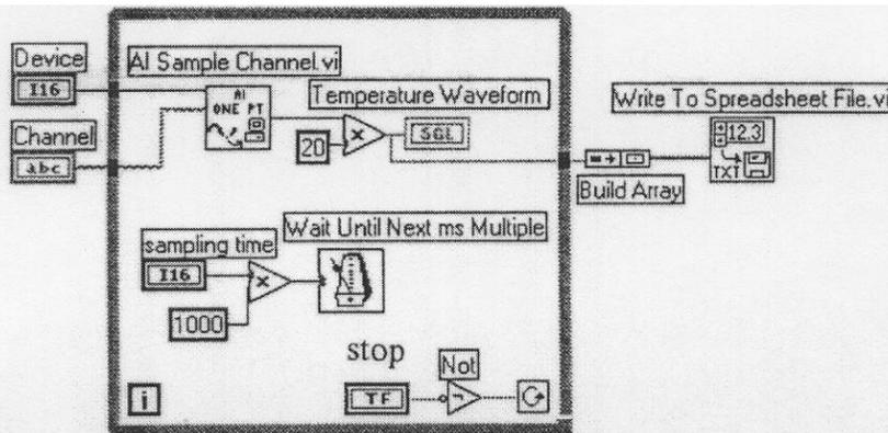
Figure 4: Block diagram for temperature measurement
