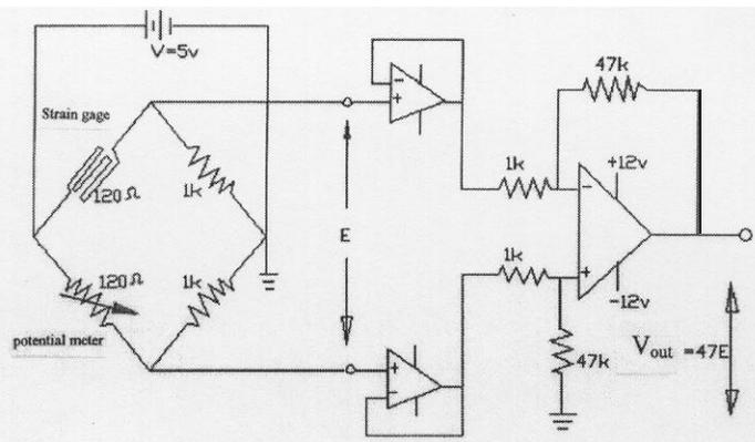
Figure 6: Circuit for stress measurement
