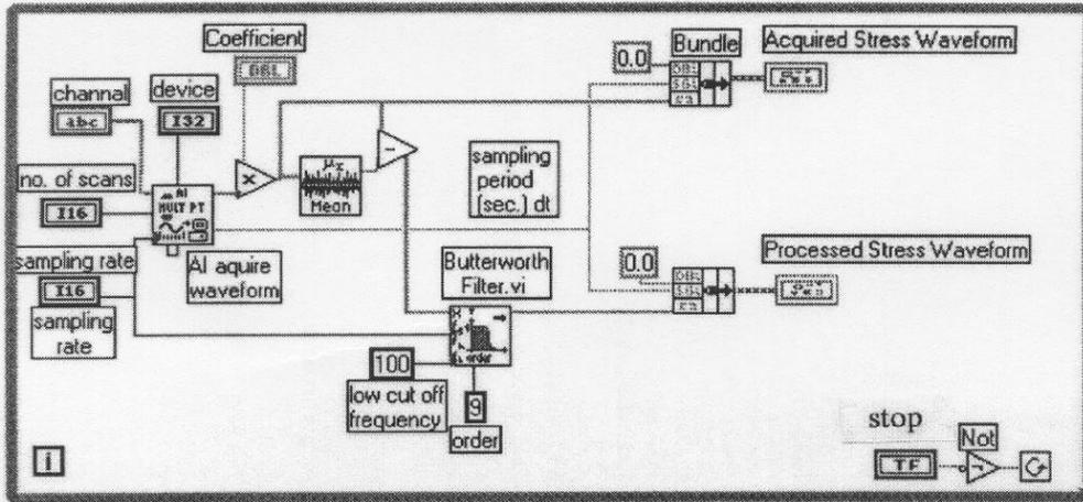
Figure 7: Block diagram for stress measurement
