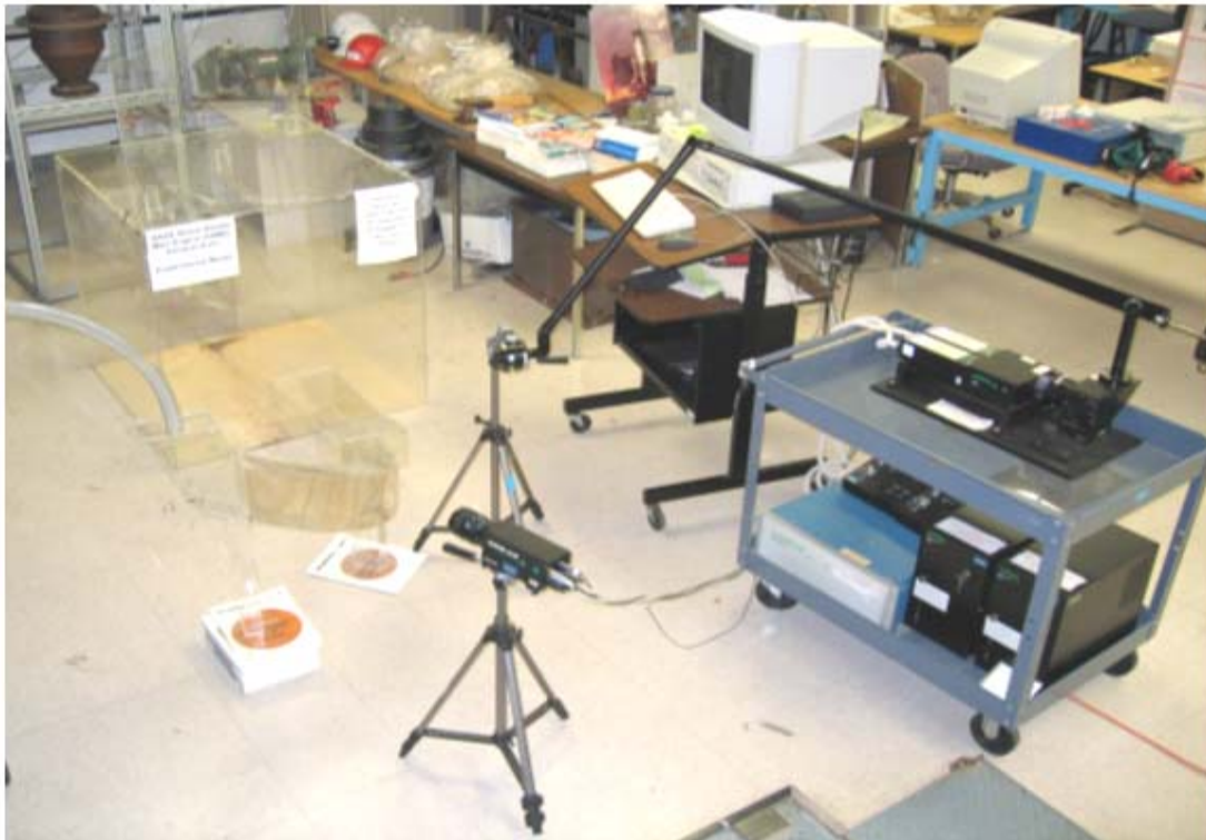
Figure A. The Pictorial View of the Experimental Model of the SSME Exhaust Duct along with the Laser-based PIV Instrumentation
