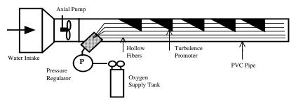
The flow past the fibers tend to induce a fluttering motion in the membrane fibers that encourages gas transfer between the fibers and the surrounding water. The fibers only occupy about 2% of the net cross sectional area of the pipe in which they are housed. When water is flowing through the module, however, the fibers are uniformly distributed throughout the section. The process provides 100% gas transfer efficiency.
