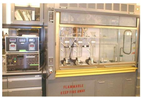
The proposed novel separation technique is electrodialysis, an electrically driven membrane separation process that is useful for removing electrolytes from solutions. This project investigates the applicability of electrodialysis to the process for production of metal compound solutions. The objectives of the project are (1) to design and build an electrodialysis unit for the separation and purification of the desired process stream, (2) to investigate the performance of electrodialysis in the
